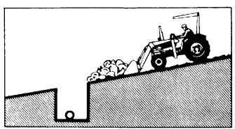
Pile dirt on the high side for easier backfilling on a slope.
